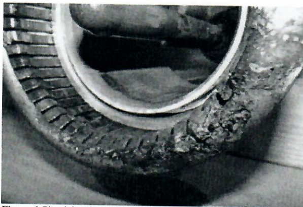
Figure 6 Circuit breaker contacts showing damage caused by electric arc
